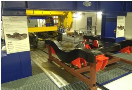
carbon fibre bogie which is due to go on initial testing early in the New Year.
